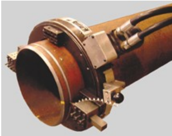
Mactech's 816 Clamshell with Sever/Bevel tooling and hydraulic drive.
